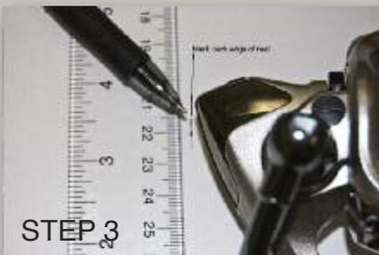
**STEP 3:** Mark the back edge of the reel. You can actually just eyeball this measurement since drop will always have an identical relationship to distance for any projected angle.
