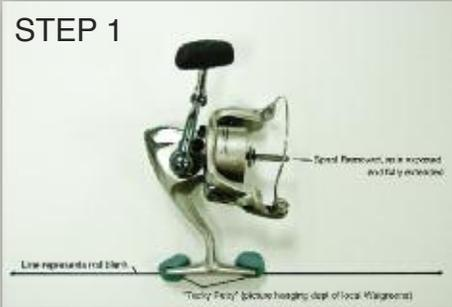
secure the foot of the reel EXACTLY on the line representing the blank (yes, we realize the reel is upside down, but we are only looking for measurements and somehow this seems easier to eyeball).
