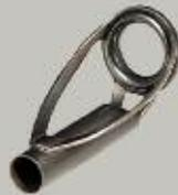
The MGTop is a medium-long tube, medium long-frame model capable of a serious contest with virtually any fish (or gunwale for that matter). Mechanically crimped and professionally braised for a lifetime of wear, the MG design features a high entry on the ring-frame braces along with Fuji's original deep pressed ring. Together these features result in unsurpassed ring retention under the worst treatment. Choose Gunsmoke SiC or Black Alconite®.
